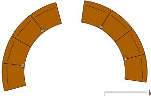
location of undermounted power outlet, typical for 2 at each piece
